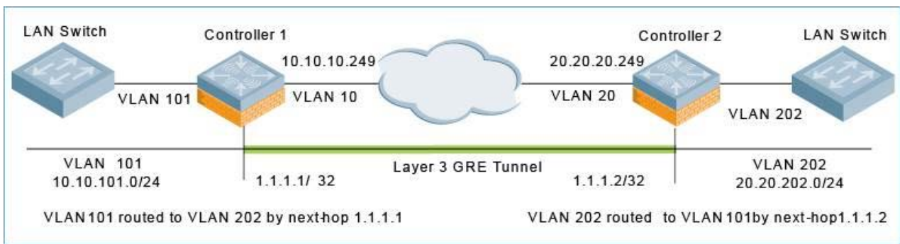
Figure 20 IPv4 Layer-3 GRE Tunnel
